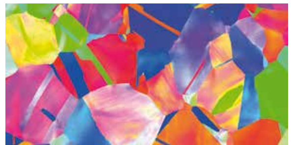
Diagram 2: IPF map showing microstructure of 6Mo stainless steel
